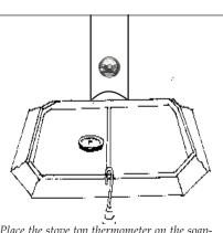
Place the stove top thermometer on the soapstone, in the center of the top of the stove, over the the catalyst, or on the first 8-10" of single wall stove pipe.
