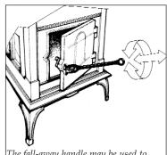
The fall-away handle may be used to operate the controls on your stove when they are too hot to handle safely.
