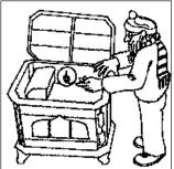
Always perform the "Match Test" before lighting your stove. If you light a match and hold it in front of the flue exit, the flame will be pulled into the flue collar if there is enough draft to light the stove.
