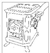
When the combustor lever is up, the combustor is in the "engaged" position. When the handle is down, the combustor is "bypassed".
